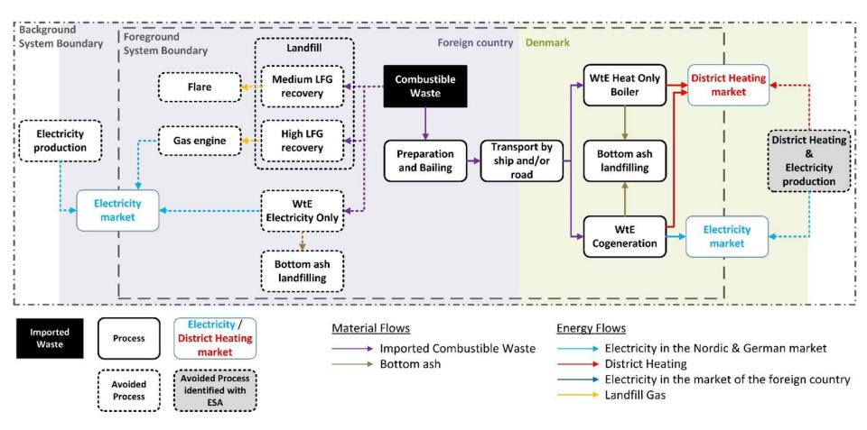
Figure 1. System boundaries, induced and avoided processes associated with import of combustible waste. The background system sitting outside a country boundary, reflect that electricity markets are international.
