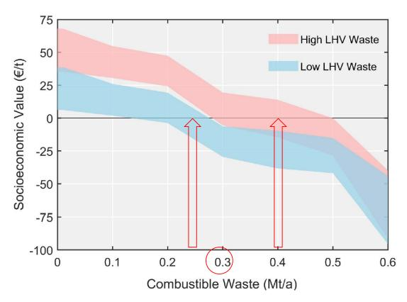
Figure 14. Uncertainty Range of the socioeconomic value from importing waste depending on the ratio between fix operational costs and variable operational costs: upper range corresponds to 35% of the waste treatment costs as variable costs and lower range corresponds to 65%
