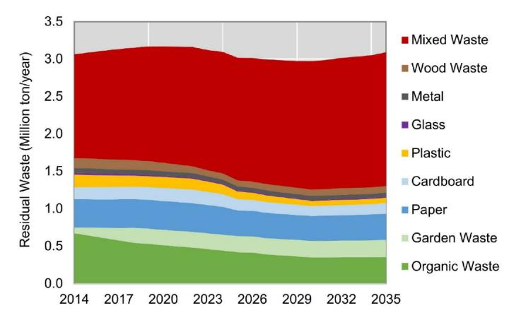
Figure 5. Forecast of household and industrial waste available for incineration in Denmark
